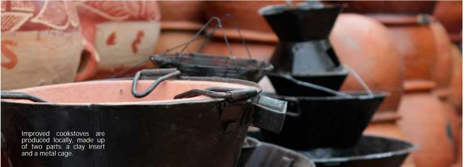
Improved cookstoves are produced locally, made up of two parts: a clay insert and a metal cage.
