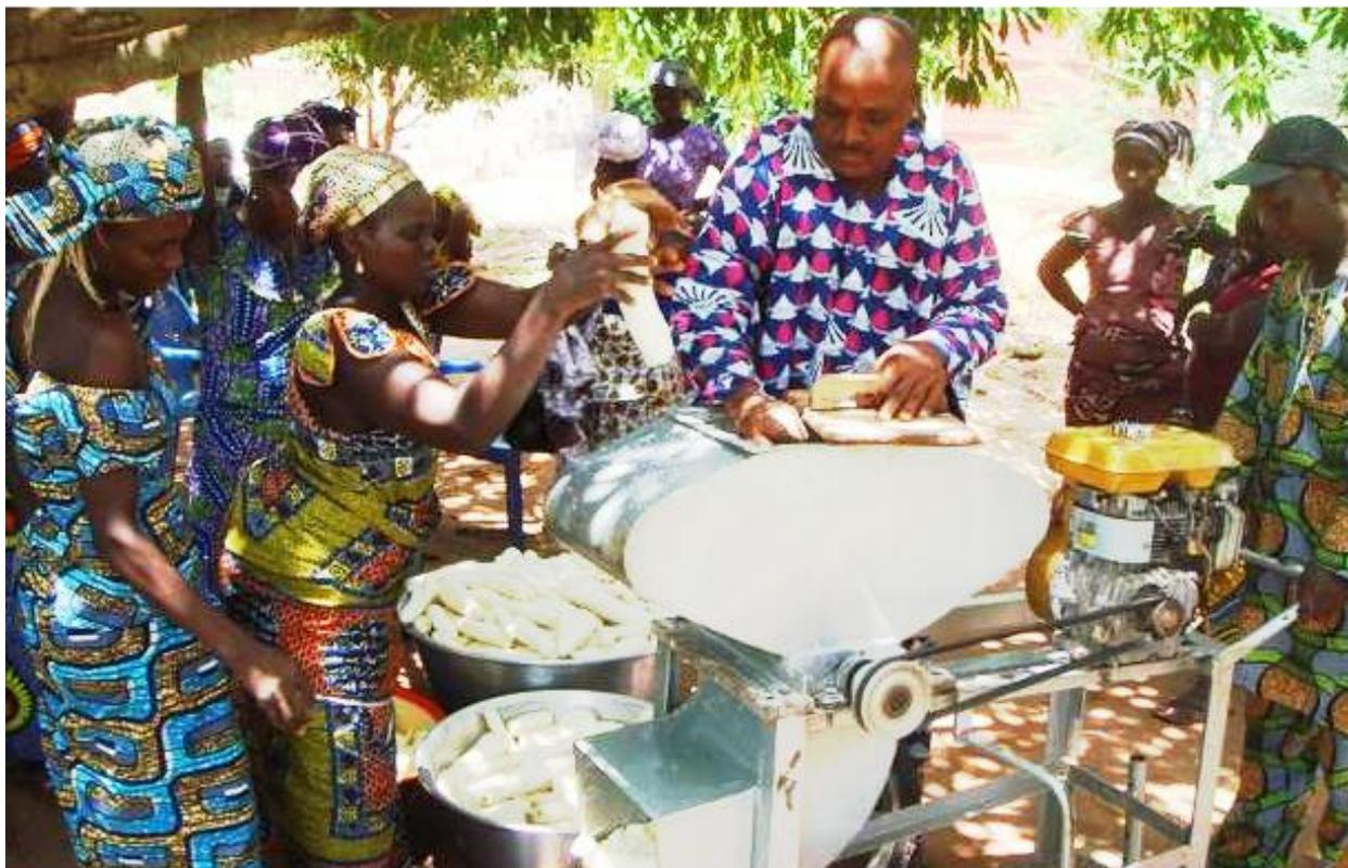
*Cassava crusher powered by a replacement jatropha-based biofuel in Benin*
