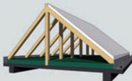
Fig 19: "Cold roof" insulation
