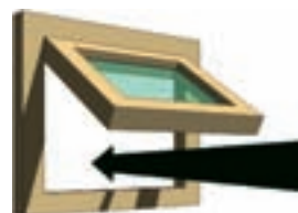
Fig 39 Outward opening windows provide efficient rain protection
