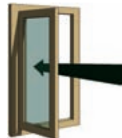
Fig 40 Outward opening vertical windows can channel the wind
