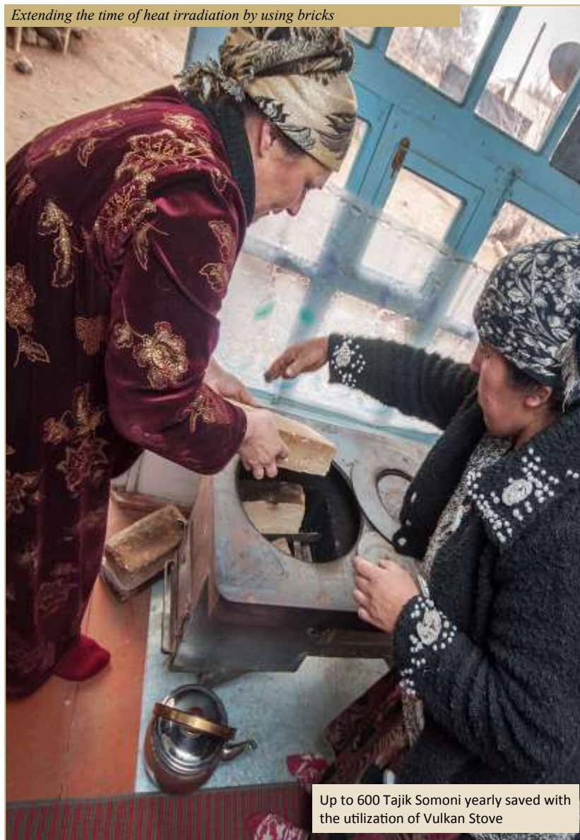
Extending the time of heat irradiation by using bricks
