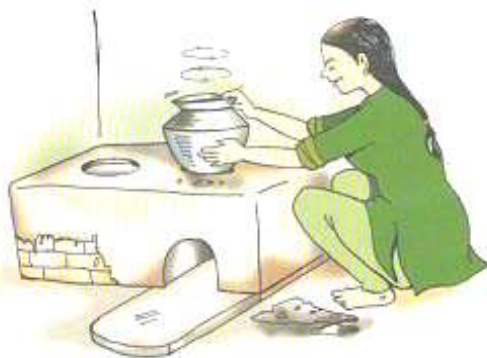
Shaping burner in the form of pot bottom
