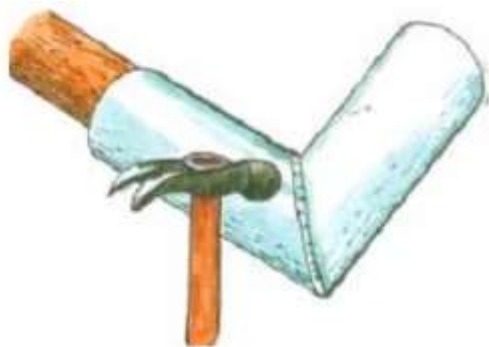
10. fastening the corner brace with short beam (log)
