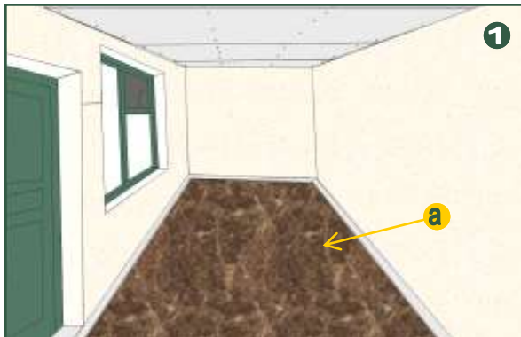
Step 1. Prepare the earthen floor (a) for insulation by cleaning the surface.
