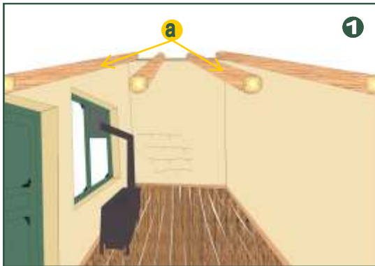
Install wooden beams (a) (15 to 20 cm) as usual.
