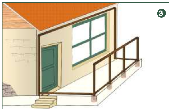
3 Then attach the beams horizontally to the lower and upper part of the columns and also between the front columns and walls.
