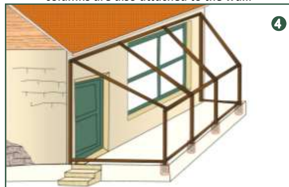
4 Place the beams on top of the horizontally assembled wood boards.
