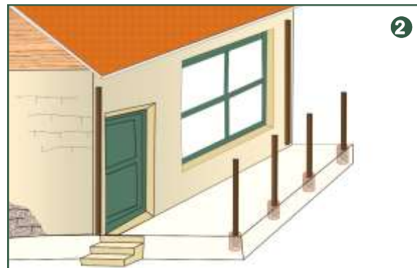
2 Install the front columns in the holes. To stabilize the columns, put stones and cement around them. Two columns are also attached to the wall.
