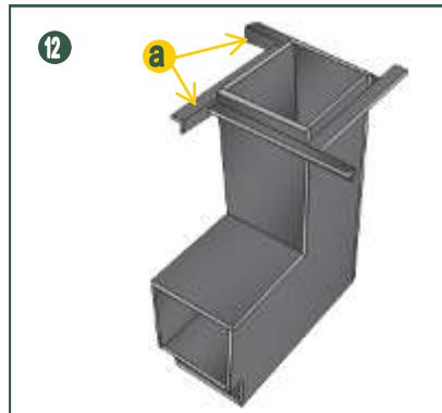
Attach 4 pieces of corner braces to the upper part of chamber wall (a) by welding
