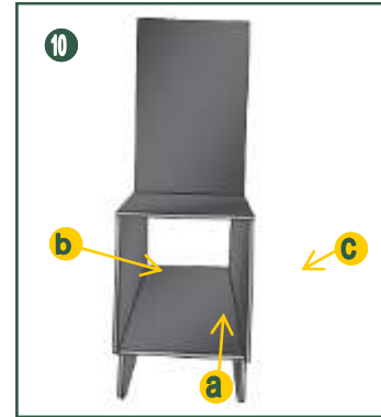
Weld the walls of lower part (a) of L shaped chamber between the left (b) and right walls (c).
