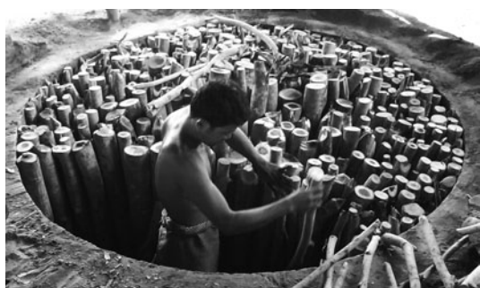
Improved charcoal kiln system, bigger and better, Cambodia.
