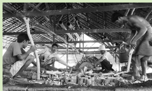
Filling an improved Yoshimura-type charcoal kiln
