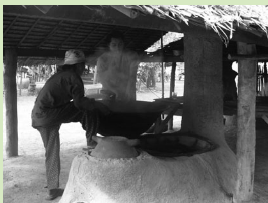
The Vattanak stove, a high-performance cooker for palm sugar making
