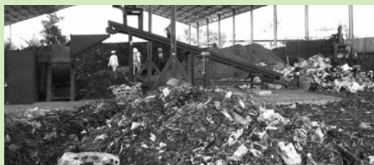
New composting facility designed for capacity to handle waste about 100 ton/day (©BALIFOKUS)
