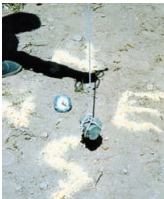
Figure 27: Finding south with a plumb line 38
