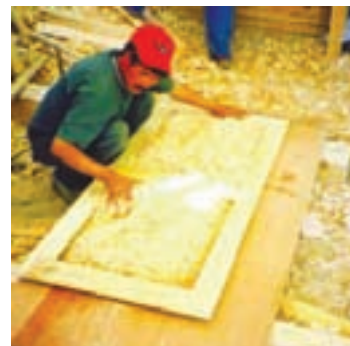
Figure 45: Assembling the door
