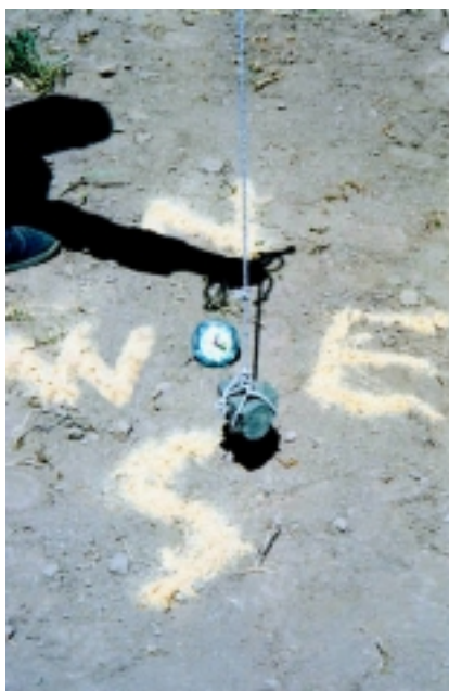
Picture 11 - View of south tracing by means of “plumb-line” method
