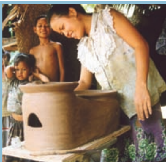
Commercial twin pot cooking stove known as the "Twin stove"
