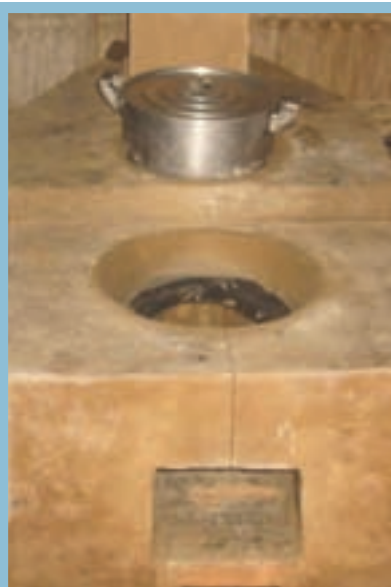
Self-built twin pot cooking stove known as the "Samaki" stove
