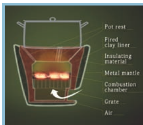
Figure 1: diagram of updraft combustion on a grate, GERES (2009)
