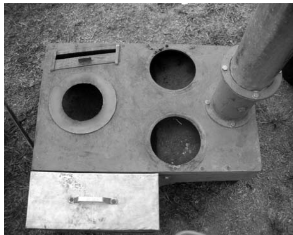
Picture of a complete improved metallic stove.
