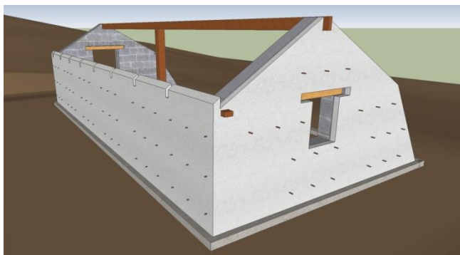
Figure 10 : Polystyrene layer installation
