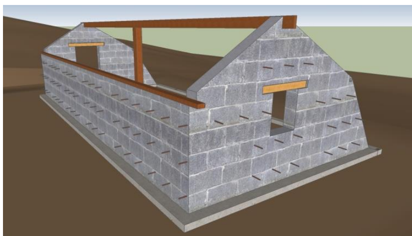
Figure 9 : Block walls, pillar and top beams and timber on north wall
